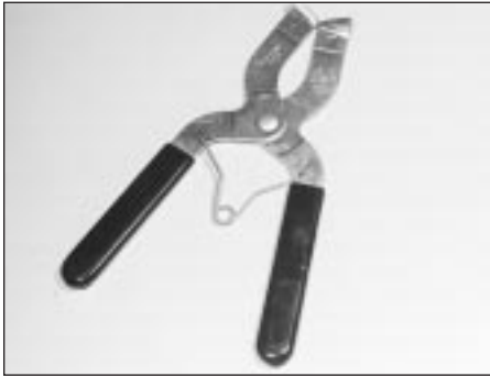
Piston ring removal/installation tool
