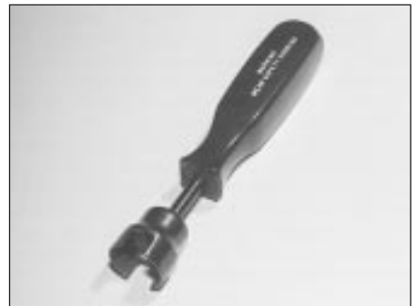
Brake shoe steady spring cup removal tool
