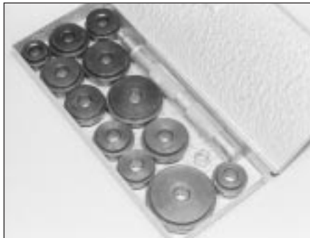
Bush and bearing removal/installation set
