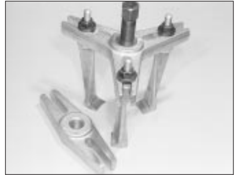
Three-legged hub and bearing puller
