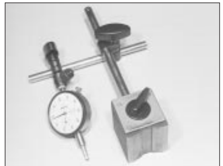
Dial test indicator and magnetic stand
