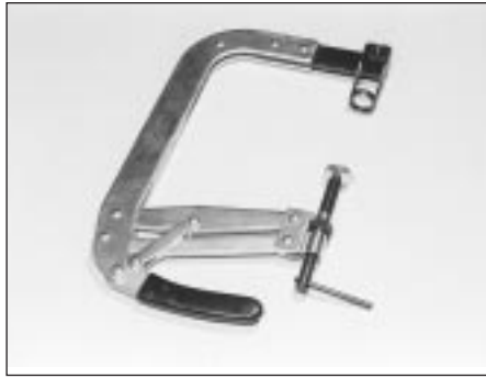
Valve spring compressor
