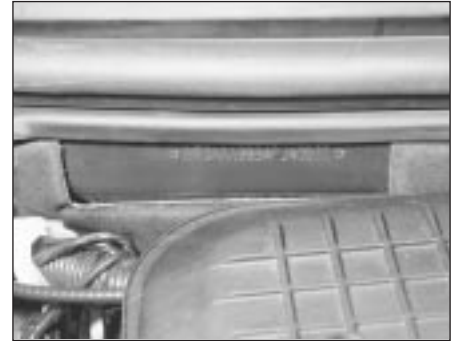
Vehicle identification number on engine compartment bulkhead
